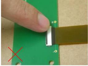
About the lock operation When you lock, it is recommended what the actuator does as a whole, and the actuator was shut surely.
