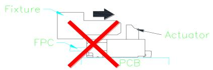
Opening the actuator by hand without using sharp tool such as tweezers.
