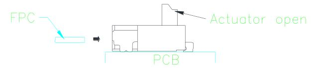
B. The actuator might not come off from the closing of the actuator in the state that FPC is not inserted and do not do, please. Do not attempt to insert the FPC if actuator is closed.
