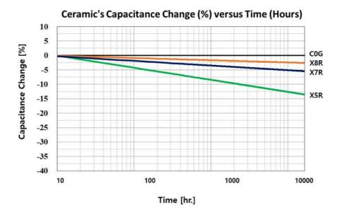
The capacitance value can be restored (also known as 'de-aged') by exposing the component to elevated temperatures approaching its curie temperature (approximately 120°C). This 'de-aging' can occur during the component's solder-assembly onto the PCB, during life or temperature cycle testing, or by baking at 150°C for about 1 hour.
