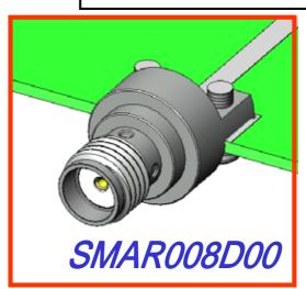
The End-launch SMA is a connector compatible with SMA (IEC60169-15). It is available in a high-performance version (SMAR006D00), which is compatible with high-frequency band up to 20GHz when mounted on the board, and a low-cost version (SMAR008D00) which is compatible with frequency up to 6GHz when mounted on the board.
