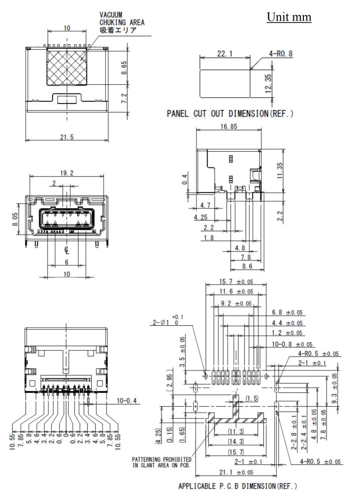
■ Socket Connector (MX62010FQ1) Drawing number: SJ113309 <u>Unit mm</u>
