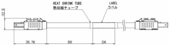
Note: In case of single end harness the opposing end will be a non-terminated pig-tail.
