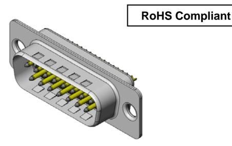
The Dsub is a typical type for highly-reliable connectors used in various electronic devices. JAE has developed the Dsub type DA-15PF-N-ME, featuring an anti-shock function with a resin insulated pin contact, for medical devices.
