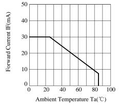
Fig.6 Forward Current Derating Curve
