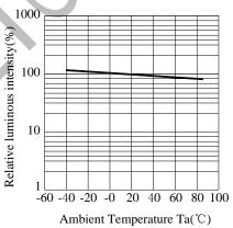
Fig.5 Luminous Intensity vs. Ambient Temperature
