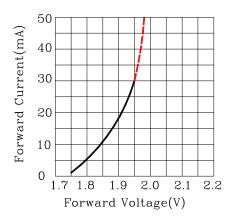
Fig.2 Forward Current vs.Forward Voltage
