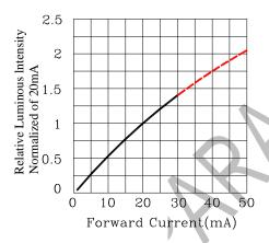
Fig.4 Relative Luminous Intensity vs.Forward Current
