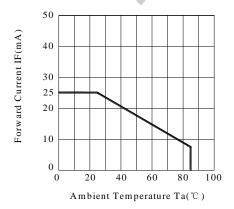
Fig.6 Forward Current Derating Curve
