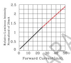
Fig.4 Relative Luminous Intensity vs.Forward Current
