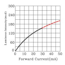
Fig.3 Luminous Intensity vs.Forward Current
