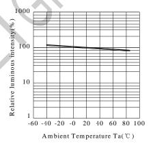
Fig.5 Luminous Intensity vs.Ambient Temperature
