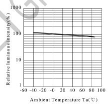
Fig.5 Luminous Intensity vs. Ambient Temperature
