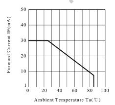
Fig.6 Forward Current Derating Curve
