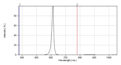
Fig.1 Super Amber Relative Intensity vs. Wavelength
