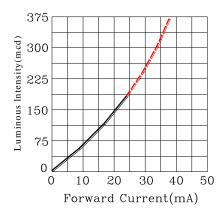
Fig.3 Luminous Intensity vs.Forward Current
