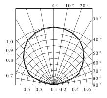
Fig.7 Relative Intensity vs.Angle
