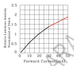
Fig.4 Relative Luminous Intensity vs.Forward Current
