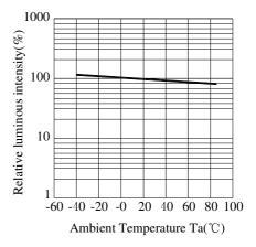
Fig.5 Luminous Intensity vs. Ambient Temperature
