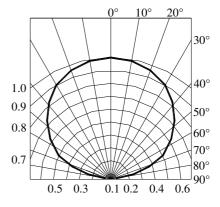
Fig.7 Relative Intensity vs.Angle
