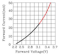
Fig.2 Forward Current vs.Forward Voltage
