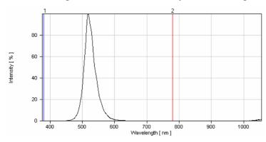
Fig.1 Green Relative Intensity vs. Wavelength
