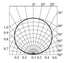
Fig.7 Relative Intensity vs.Angle
