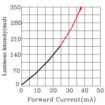
Fig.3 Luminous Intensity vs.Forward Current
