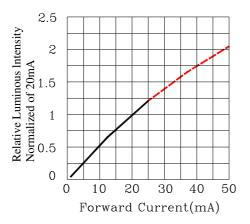
Fig.4 Relative Luminous Intensity vs.Forward Current
