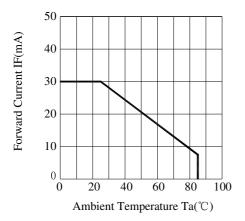
Fig.6 Forward Current Derating Curve
