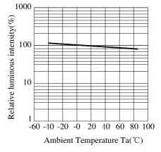
Fig.5 Luminous Intensity vs. Ambient Temperature
