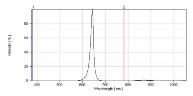
Fig.1 Red Relative Intensity vs. Wavelength
