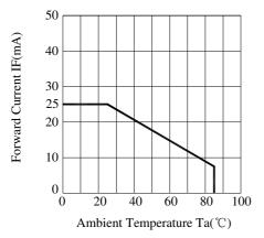
Fig.6 Forward Current Derating Curve
