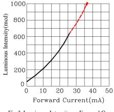
Fig.3 Luminous Intensity vs.Forward Current
