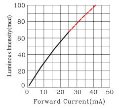
Fig.3 Luminous Intensity vs.Forward Current
