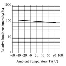
Fig.5 Luminous Intensity vs.Ambient Temperature
