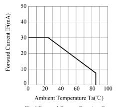
Fig.6 Forward Current Derating Curve
