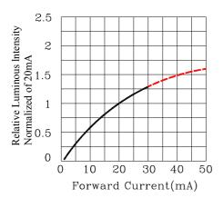
Fig.4 Relative Luminous Intensity vs.Forward Current
