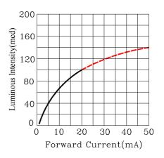
Fig.3 Luminous Intensity vs.Forward Current
