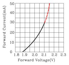
Fig.2 Forward Current vs.Forward Voltage
