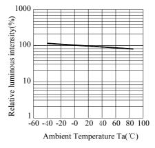
Fig.5 Luminous Intensity vs. Ambient Temperature
