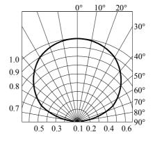
Fig.7 Relative Intensity vs.Angle
