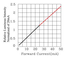
Fig.4 Relative Luminous Intensity vs.Forward Current
