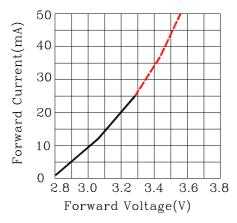
Fig.2 Forward Current vs.Forward Voltage
