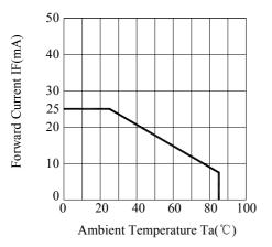
Fig.6 Forward Current Derating Curve
