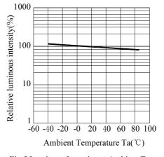
Fig.5 Luminous Intensity vs. Ambient Temperature
