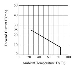
Fig.6 Forward Current Derating Curve
