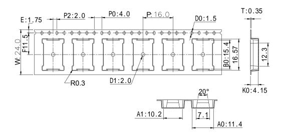
Note: Tolerances unless mentioned ±0.25mm. Unit = mm
