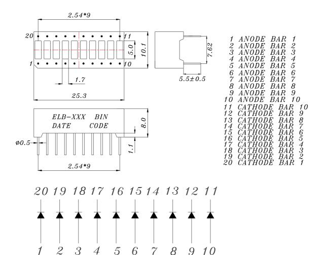
Note: Tolerances unless mentioned  $\pm 0.25$ mm. Unit = mm
