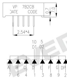
Note: Tolerances unless mentioned ±0.25mm. Unit = mm
