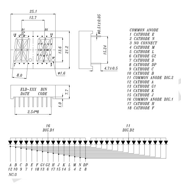
Note: Tolerances unless mentioned ±0.25mm. Unit = mm
