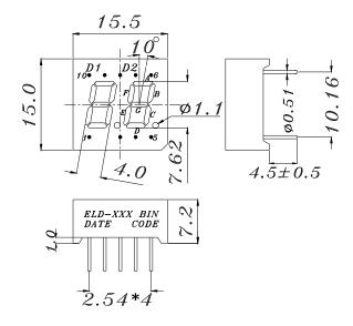
COMMON ANODE CATHODE GNO PIN3 CATHODE A CATHODE F5 COMMON ANODE D2 6 CATHODE D7 CATHODEE8 CATHODE CCATHODE9 10 COMMON ANODE D1
