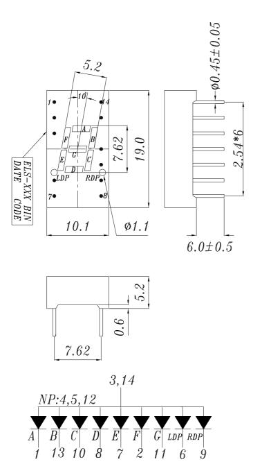
COMMON ANODE 1 CATHODE A 2 CATHODE F 3 COMMON ANODE 4 NO PIN 5 NO PIN 6 CATHODE LDP 7 CATHODE LDP 7 CATHODE D 9 CATHODE RDP 10 CATHODE RDP 10 CATHODE C 11 CATHODE G 12 NO PIN 13 CATHODE B 14 COMMON ANODE
