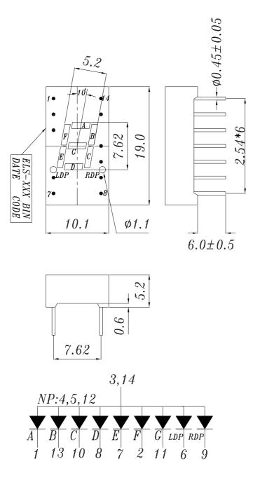
COMMON ANODE 1 CATHODE A 2 CATHODE F 3 COMMON ANODE 4 NO PIN 5 NO PIN 6 CATHODE LDP 7 CATHODE LDP 7 CATHODE E 8 CATHODE D 9 CATHODE RDP 10 CATHODE C 11 CATHODE C 12 NO PIN 13 CATHODE B 14 COMMON ANODE
