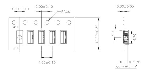
Note: Tolerances unless mentioned ±0.1mm. Unit = mm
