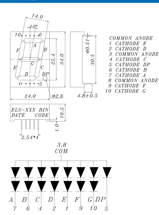
Note: Tolerances unless mentioned ±0.25mm. Unit = mm
