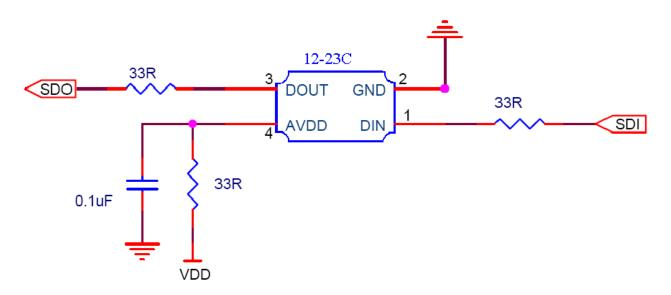
When 12-23C is set to operate on 5V power system, a 0.1uF capacitor is recommended to add between power supply and ground terminal. The capacitor is suggested to put as closer as possible to IC position. There are frequent resistors were used on different drain voltage as listed table.
