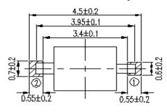
Note: The tolerances unless mentioned are ±0.1, unit=mm.
