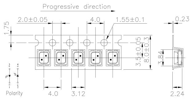
Note: Tolerances unless mentioned ±0.1mm. Unit = mm
