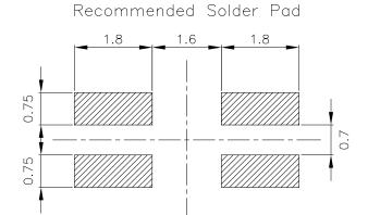
Note: Tolerances unless mentioned ±0.1mm. Unit = mm
