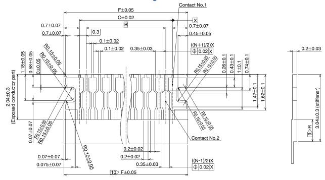
Note 9 When designing the FPC dimension R must be 0.5mm minimum.
