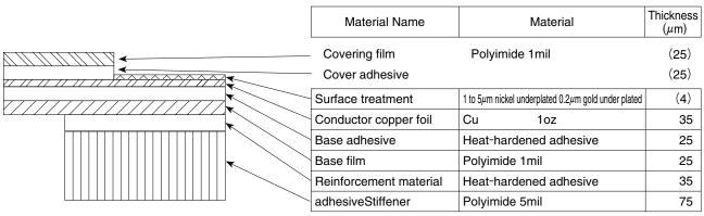
Note 1. Material composition of FPC is a reference example. Please adjust the thickness of the FPC mating section to 0.2±0.03mm in reference to the material composition.
