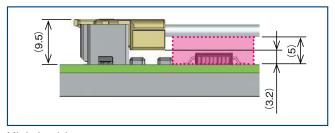
Minimized keep-out space Other components can be mounted under the cables
