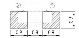
Note: Tolerances unless mentioned ±0.1mm. Unit = mm Suggested pad dimension is just for reference only. Please modify the pad dimension based on individual need.
