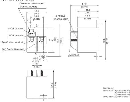
>>> Wiring Diagram (Top view)
