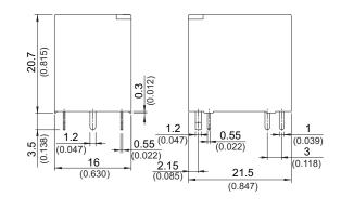
$\begin{array}{c} \mbox{TOLERANCE:} \\ \mbox{LESS THAN:} & 1(0.039) \pm 0.1(0.004) \\ & 5(0.197) \pm 0.3(0.012) \\ & 20(0.787) \pm 0.5(0.020) \\ \mbox{MORE THAN:} & 20(0.787) \pm 1(0.039) \end{array}$
