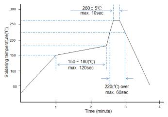
Recommended IR Reflow Soldering Profile
