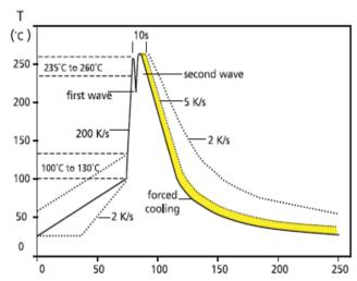
Recommended double-wave Soldering Profile Typical values (solid line)
