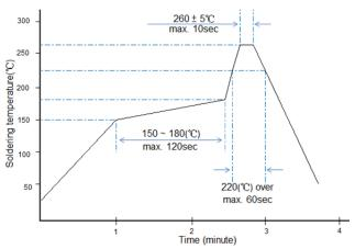
Recommended IR Reflow Soldering Profile MEET J-STD-020D
