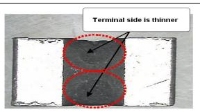
8.2.2 When customer performs wave solder process shall take note on the dispensing gap. If the gap between two dispensing is over, the red-glue will not adhesive the resistor body and be dropped out (as photo 1). Therefore, we suggest customer to narrow down the dispenser gap (as photo 2), or dispenser on the body center (as photo 3)
