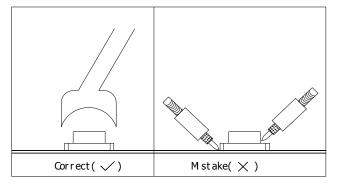
Avoid rubbing or scraping the resin by any object, during high temperature, for example reflow solder etc.
