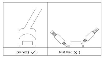
■ Avoid rubbing or scraping the resin by any object, during high temperature, for example reflow solder etc.
