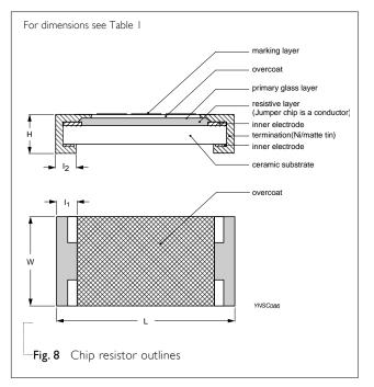
Chip Resistor Surface Mount AF SERIES 0100 to 2512
