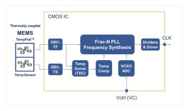
Figure 22. Block Diagram - VCTCXO
