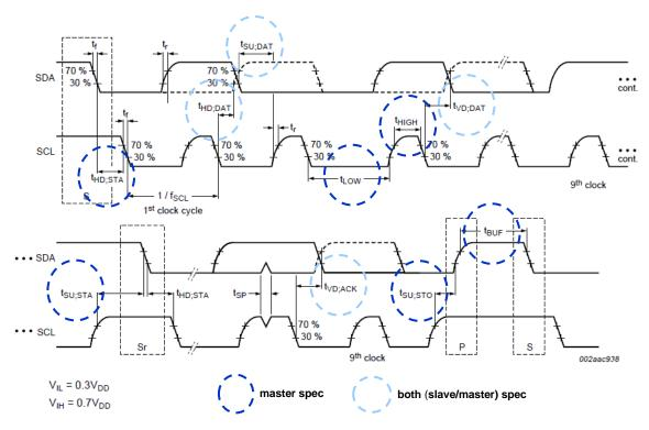
Figure 35. I<sup>2</sup>C Timing Diagram
