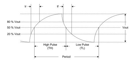
Figure 15. Clipped Sinewave Waveform Diagram
