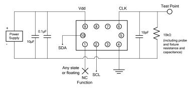
Figure 13. Clipped Sinewave Test Circuit (1<sup>2</sup>C Control)
