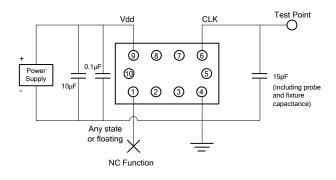
Figure 10. LVCMOS Test Circuit (NC Function)
