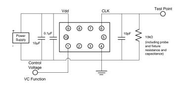
Figure 9. Clipped Sinewave Test Circuit (VC Function)
