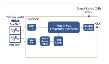
Figure 20. Block Diagram - TCXO
