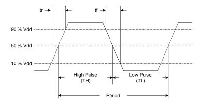
Figure 14. LVCMOS Waveform Diagram
