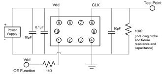
Figure 6. LVCMOS Test Circuit (OE Function)
