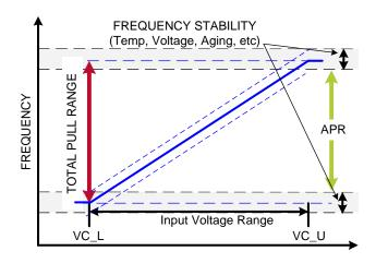
Figure 26. Typical SiTime VCTCXO FV Characteristic
