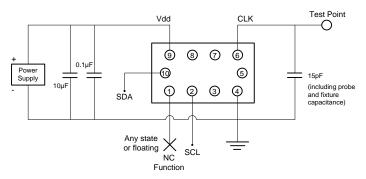
Figure 12. LVCMOS Test Circuit (I<sup>2</sup>C Control)
