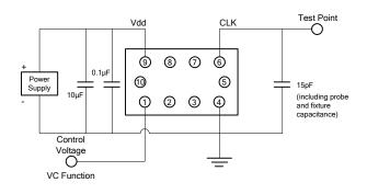
Figure 8. LVCMOS Test Circuit (VC Function)
