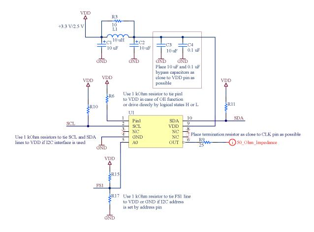
Figure 36. Schematic Example - DCTCXO
