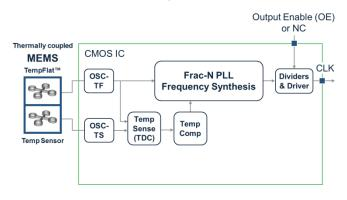
Figure 36. Block Diagram – TCXO
