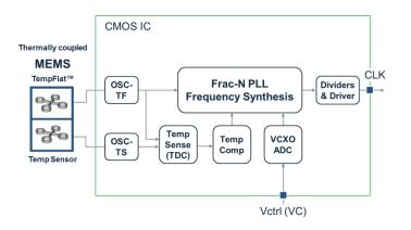
Figure 37. Block Diagram – VCTCXO
