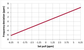
Figure 27. DCTCXO frequency pull characteristic
