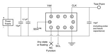
Figure 12. LVCMOS Test Circuit (I<sup>2</sup>C Control), DCTCXO mode
