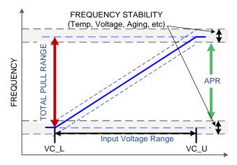
Figure 41. Typical SiTime VCTCXO FV Characteristic
