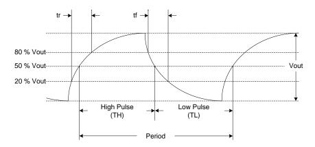
Figure 16. Clipped Sinewave Waveform Diagram<sup>[11]</sup>
