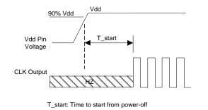
Figure 17. Startup Timing
