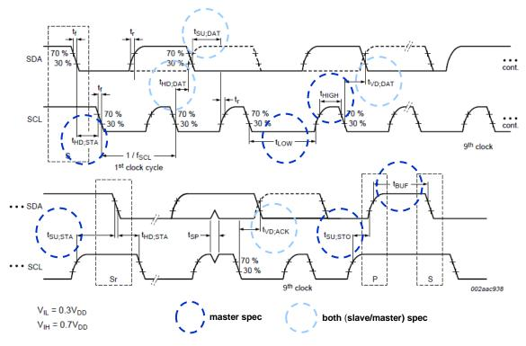
Figure 48. I<sup>2</sup>C Timing Diagram
