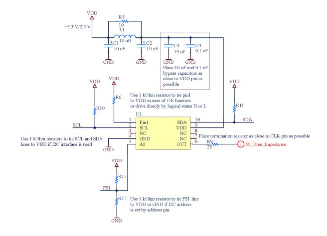
Figure 49. DCTCXO schematic example.
