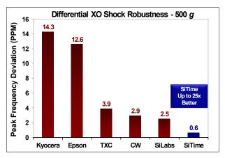
Figure 6. Shock Robustness<sup>[6]</sup>
