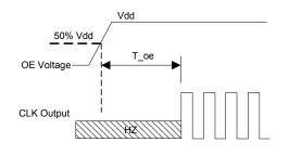
T\_oe: Time to re-enable the clock output
