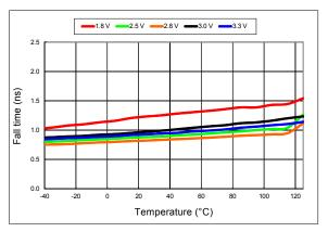
Figure 13. 20%-80% Fall Time vs Temperature
