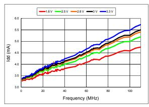
Figure 8. Idd vs Frequency
