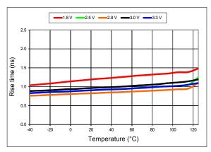
Figure 12. 20%-80% Rise Time vs Temperature
