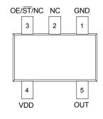
Figure 1. Pin Assignments
