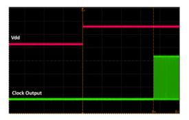
Figure 17. Startup Waveform vs. Vdd
