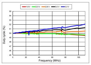
Figure 11. Duty Cycle vs Frequency
