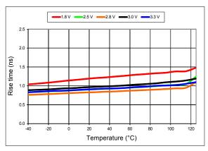
Figure 12. 20%-80% Rise Time vs Temperature
