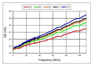
Figure 8. Idd vs Frequency
