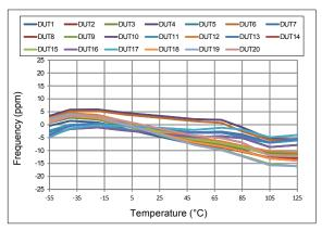
Figure 9. Frequency vs Temperature
