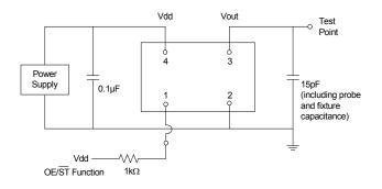
Figure 2. Test Circuit
