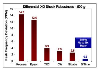
Figure 6. Shock Robustness<sup>[6]</sup>
