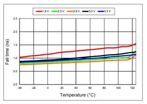
Figure 13. 20%-80% Fall Time vs Temperature
