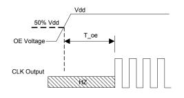
T\_oe: Time to re-enable the clock output
