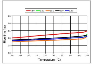
Figure 12. 20%-80% Rise Time vs Temperature
