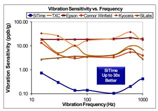
Figure 5. Vibration Robustness<sup>[5]</sup>
