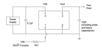
Figure 2. Test Circuit
