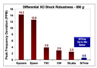
Figure 6. Shock Robustness<sup>[6]</sup>
