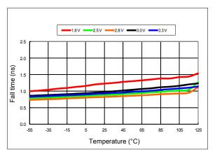
Figure 13. 20%-80% Fall Time vs Temperature
