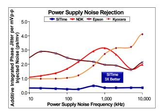
Figure 4. Power Supply Noise Rejection<sup>[4]</sup>
