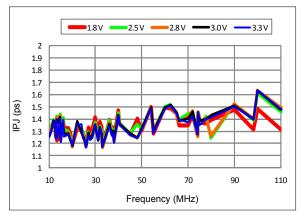
Figure 14. RMS Integrated Phase Jitter Random (12 kHz to 20 MHz) vs Frequency<sup>[11]</sup>
