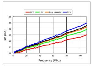
Figure 8. Idd vs Frequency
