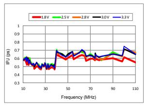
Figure 15. RMS Integrated Phase Jitter Random (900 kHz to 7.5 MHz) vs Frequency<sup>[11]</sup>
