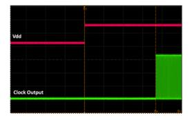
Figure 17. Startup Waveform vs. Vdd
