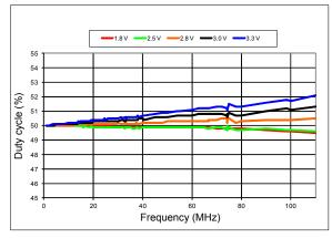
Figure 11. Duty Cycle vs Frequency
