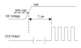
Figure 6. OE Enable Timing (OE Mode Only)
