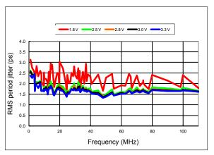
Figure 10. RMS Period Jitter vs Frequency
