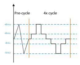
Figure 1: Pre-conditionning differential current cycles
