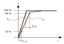
Figure 2:  $t_{\rm D\,10}$  (delay time @ 10 %) and  $t_{\rm D\,90}$  (delay time @ 90 %)
