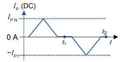
Figure 1: Current cycle used to measure magnetic and electrical offset (transducer supplied)
