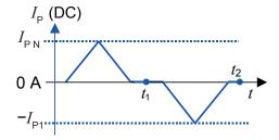
Figure 14: Current cycle used to measure magnetic and electrical offset (transducer supplied)
