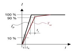
Figure 16: Response time  $t_{\rm r}$  and reaction time  $t_{\rm ra}$
