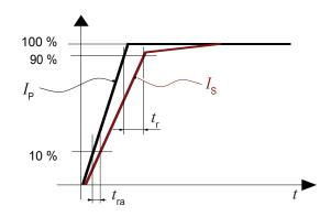
Figure 6: Response time  $t_{\rm r}$  and reaction time  $t_{\rm ra}$
