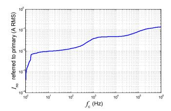
Figure 4: Typical total output RMS noise current with  $R_{\rm M}$  = 100  $\Omega$  (primary referred)
