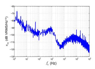
Figure 3: Typical output noise voltage spectral density  $e_{\rm no}$  with  $R_{\rm M}$  = 100  $\Omega$
