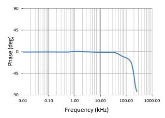
Figure 5: Typical frequency response, small signal bandwidth
