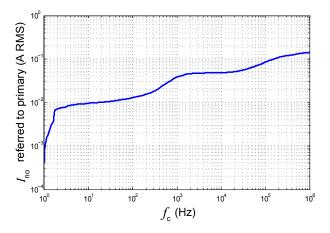
Figure 4: RMS noise current referred to primary  $I_{no}$ with  $R_{M}$  = 100  $\Omega$
