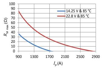
Figure 1: Maximum measuring resistance
