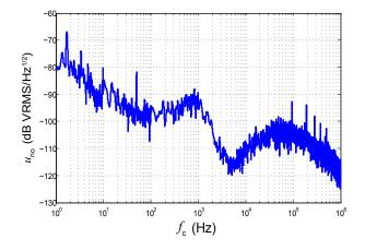
Figure 3: Noise voltage spectral density referred to primary  $u_{no}$  with  $R_{\rm M}$  = 100  $\Omega$
