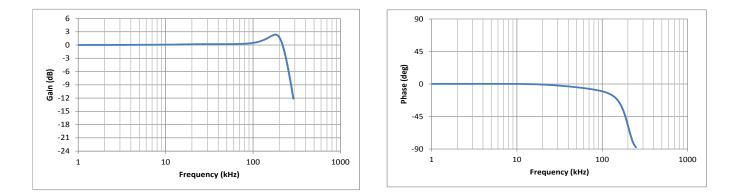
Figure 5: Typical frequency response, small signal bandwidth
