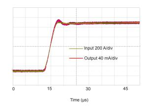
Figure 2: Typical step response (0 to 1 kA, 200 A/µs)
