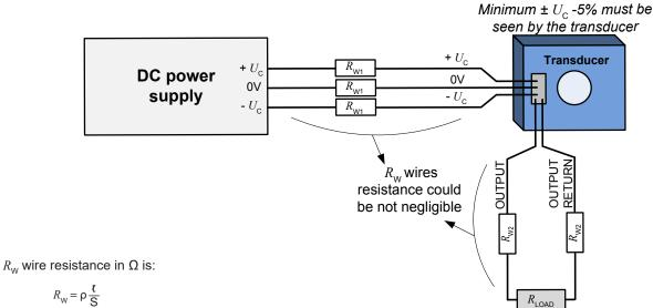
Cross section of wire in m<sup>2</sup> S:
