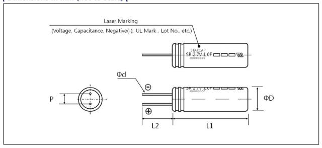
Note: It is not allowed to go through reflow (IR, Atmosphere heating methods etc.) process
